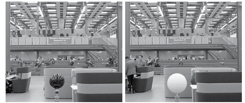
Fig · 5 A black shiny probe and a matte white probe. Both were photographed in the same light. Note that they bring out different light qualities.
